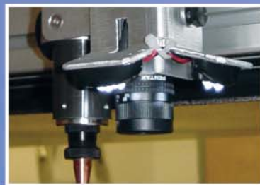
High performance cutting head with integrated i-laser ™ CCD vision system
